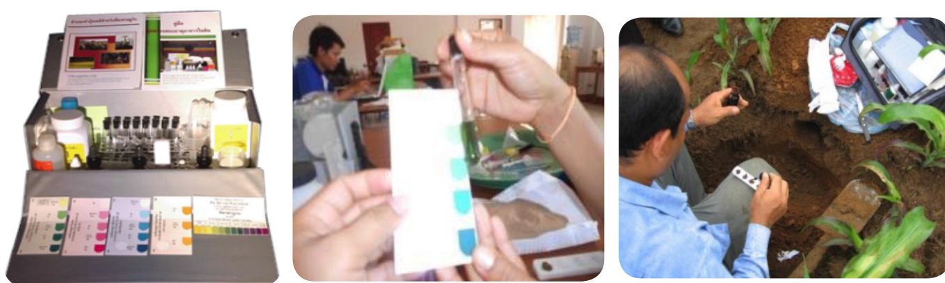
Photo 19 Soil analysis using soil test kit
