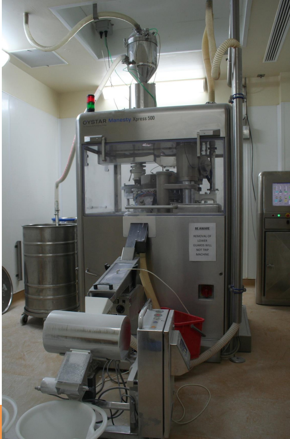
Example of a tablet press and its ancillary equipment placed in an isolated area
