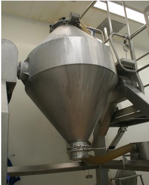
A double-cone powder mixer (tumble blender)
