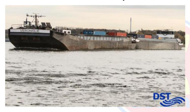
Coupled Formation: GMS Veronique, L: 110.00 m – B: 11.45 m – D: 3.32 m – T: 3066 t / 208 TEU – P: 2 x 970 kW + 300kW bow thruster; Barge VERONIQUE II, L: 71.00 m – B: 11.45 m – P: approx. 560 kW + 240 kW bow thruster
