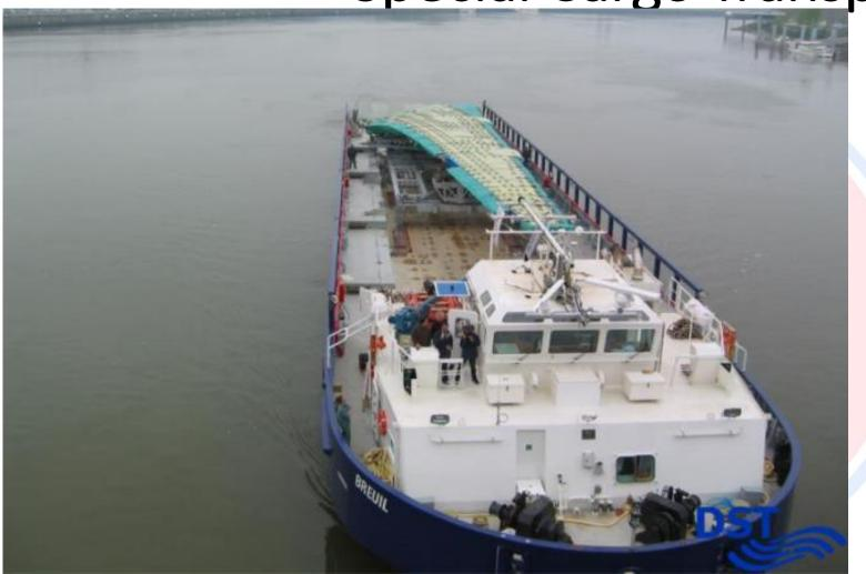
Motor vessel for special heavy or voluminous cargo: Roro BREUIL, L: 75.0 m – B: 13.8 m – T: 1300t. The BREUIL carries the wings for the Airbus A380.
