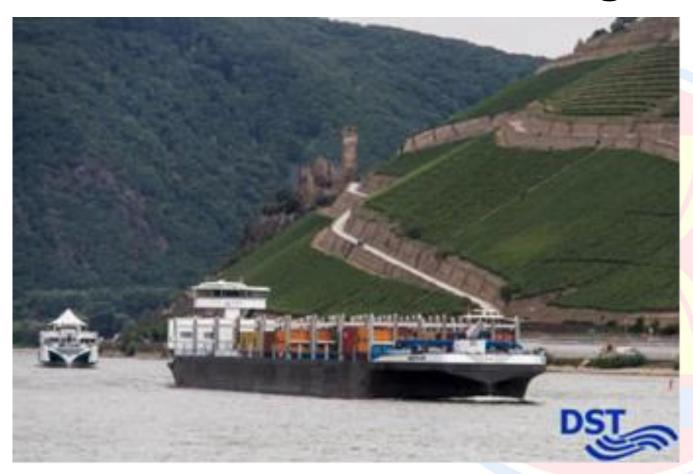
Container ship: GMS NOVA, L: 134,16m – B: 16,90m – D: 3,52m – T: 5175t – P: 2 x 1100kW + 860kW and 400kW bow thrusters
